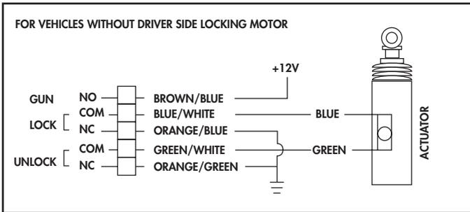
This system has a switch instead of an actuator in the drivers door. You will need to mount an actuator (GT series) in the drivers door to control your locks. Wiring diagram comes with actuator (GT series)
