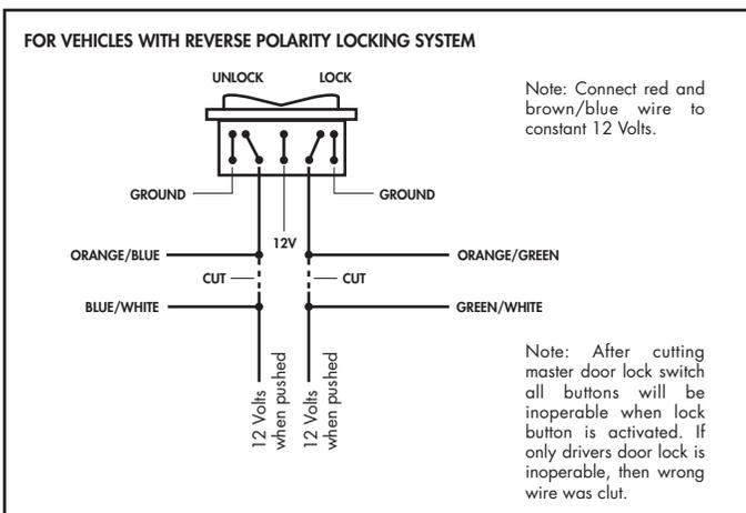
Similar to positive trigger, but will have 5 wires. 2 wires will be grounded, another 2 wires will be positive triggers, and 1 will have a constant 12 volts (sender wire).
