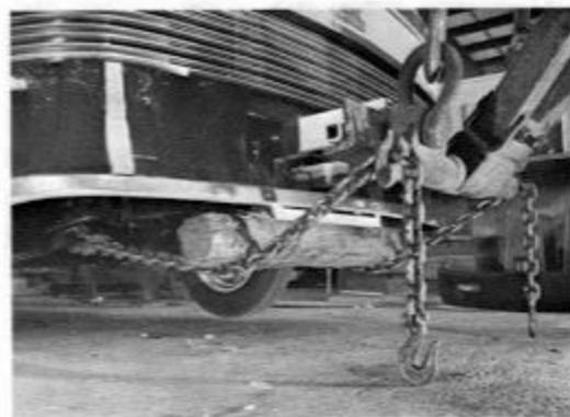
8. Wood beam inserted into horizontal support channel.
