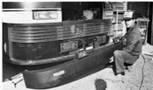
3. Remove both front bumper bracket support plates. Retain the bumper bracket support bolts for use on the tow package.
