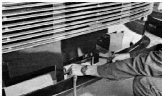
5. Install the frame extension rails with the cross tube receptacle in the down position.
