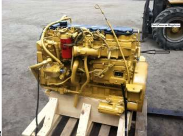
C12 Engine (C9 regulator in same location)
