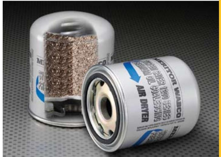
For best efficiency and to ensure the air system remains clean, replace the coalescing desiccant cartridge every 2 years or 200,000 miles or more often, depending on usage, vocation and condition of the compressor. The air system should be checked weekly for moisture. If moisture is found, replace the desiccant cartridge.
